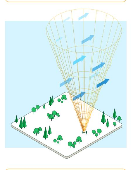
Allows measurements to be taken up to 300 metres in height.
