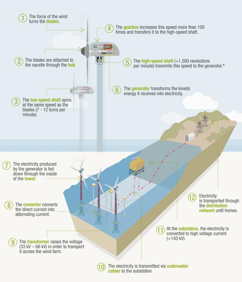
(\*) Some technologies use low-speed generators coupled directly to the low-speed shaft.
