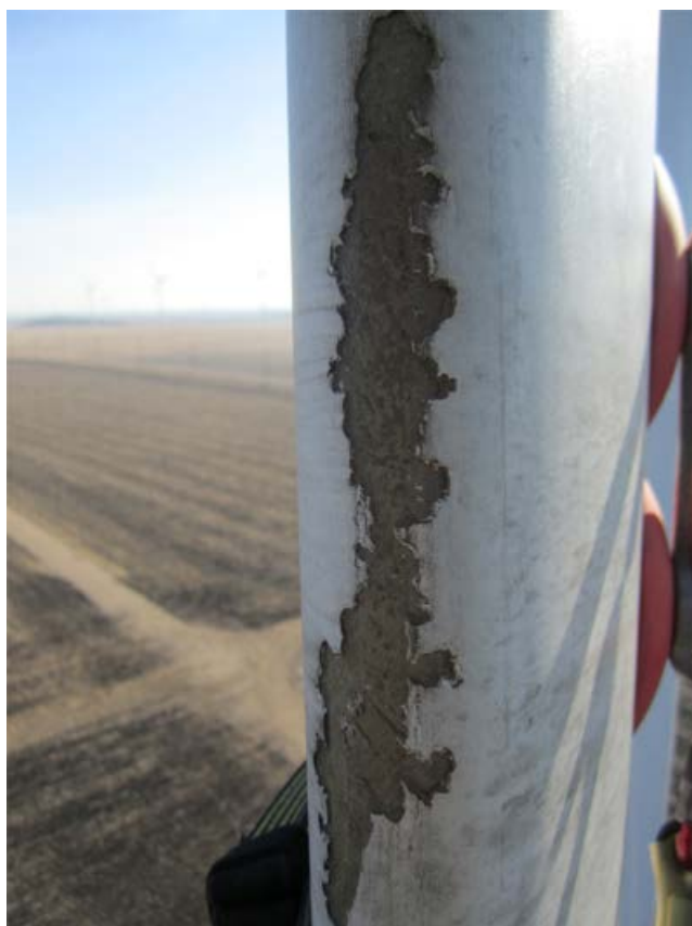
Leading edge erosion on a wind turbine blade [Source: North America Clean Energy website]
