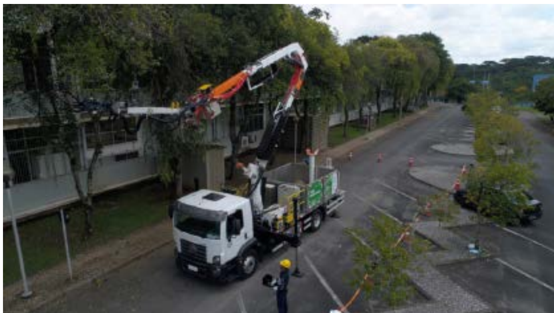
Truck with robotic system with extensible arm coupled
