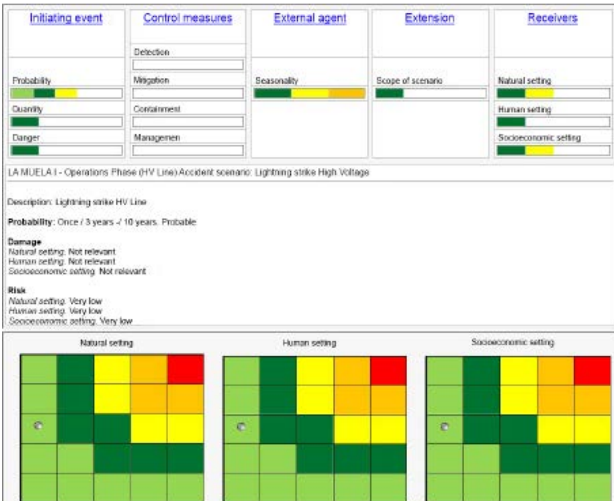
Example of the information shown by the ARIAN tool when the accident 'Lightning strike in an HV line in Wind Farm 1' is selected. The result of the risk calculation is Very Low for all environments, as shown by the risk matrices (marker in green zone), which also show that the scenario is probable (probability=3) and the damage is Not Relevant.
