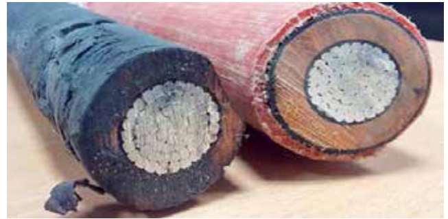
Cable cross-cut with two different degrees in ageing
