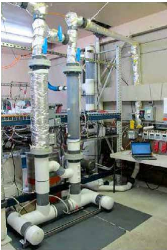
Macrofouling control process employing CO 2
