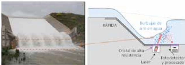
Example of optical air bubble sensor application in a dam
