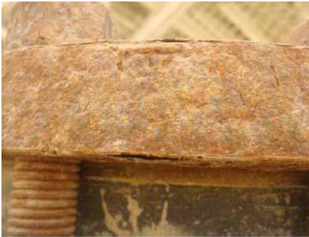
Generalised corrosion on bolts and flange, Mesaieed CC
