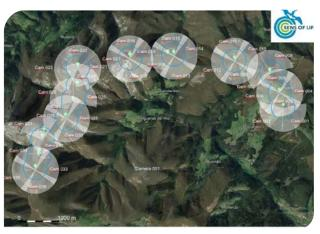
Modeling the volume monitored by the cameras for a bird with a wingspan of 150cm.
